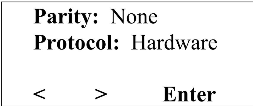
This menu allows you to change the serial port setting by change the Parity and Handshaking Protocol. You must make sure that this setting and the setting at host computer match.
