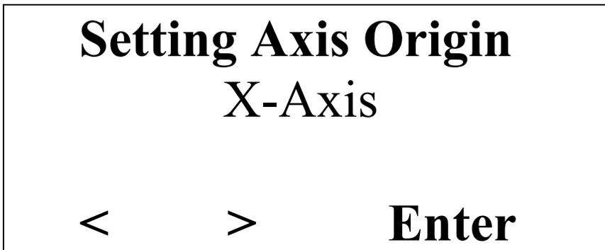
This menu allows you to set the current axis position to be the origin. You can set axis origin individually or all axis at once.
