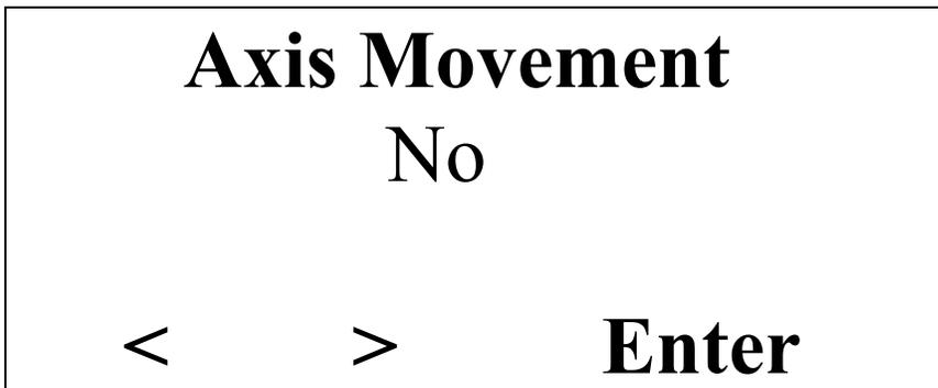
This menu allows you to move one axis at a time either in absolute or relative mode. By selecting Yes, it will take you to a sub menu where you can select what axis to move and what mode to move (Absolute or Relative).
