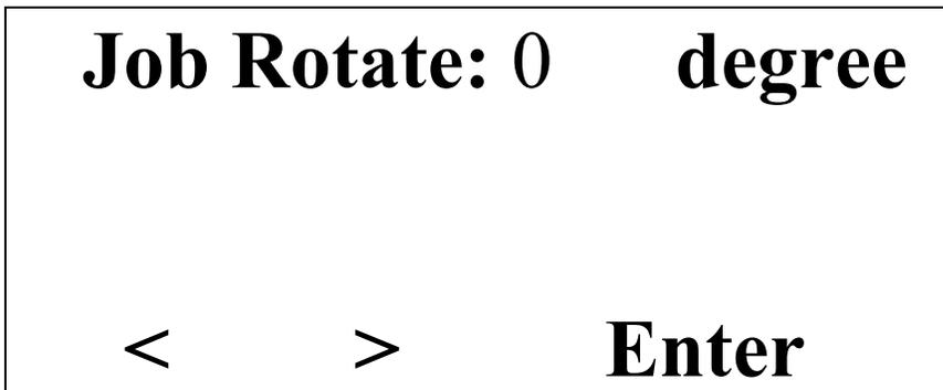
This menu allows you to rotate the job from 0 to 90 degree.
