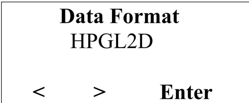
This menu allows you to select a different data format. The data format is depending on the software you are using in driving our router.
