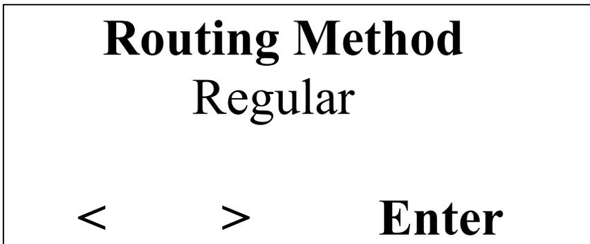
This menu allows you to change the method of routing from Regular route to Contour route. If the Contour method is selected, sub menu will be displayed to enter registration points.
