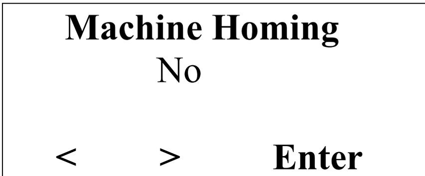
This menu allows you to home the machine. Homing is the same as move all axis to machine origin.
