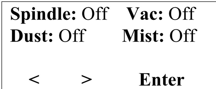
This menu allows you to turn on/off individual devices. The displayed status of the devices is the current status of that device.
