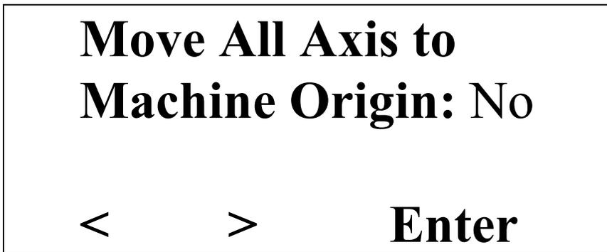
This menu allows you to move all axis to the machine origin which is the position after machine powered up. As soon as the Yes selection is confirmed, all axis will be moving to the machine origin.
