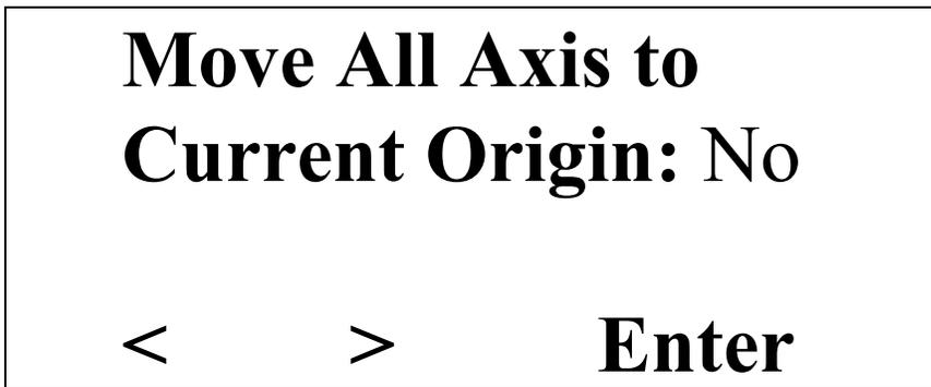
This menu allows you to move all axis to the current origin which is the positions after you set in the Setting Axis Origin or the origin currently saved in the default. As soon as the Yes selection is confirmed, all axis will be moving to the current origin.
