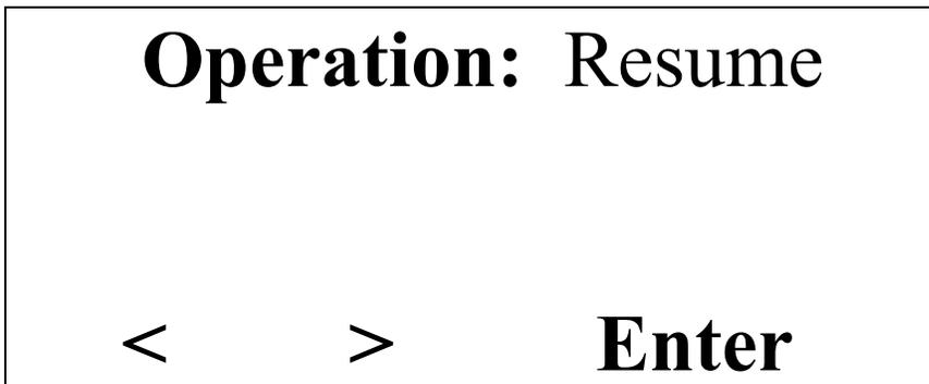
This menu will be prompted whenever the machine is in pause mode. It allows you to resume or abort the routing operation
