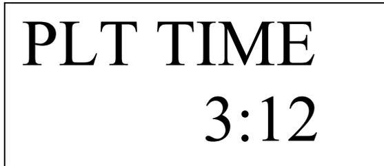
This screen display how many hours and minutes cutter/plotter has been cutting/drawing.
