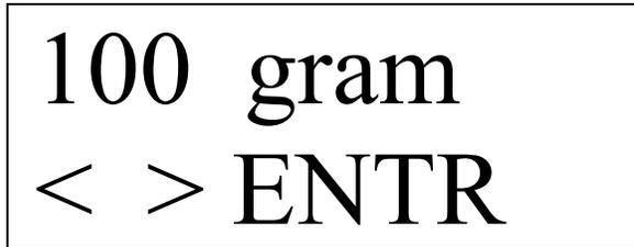
This menu allows you to change the cutting pressure of the cutting head between 30-400 grams (1-14 ounces). You can change the tool pressure while the plotter is plotting as well as while it is not plotting. Tool pressure setting sent by your computer software may override setting made at the keypad.
