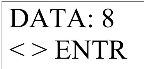
This menu will allow you to change the “DATA” bits of the plotter communications to match the software communication protocol. This menu is only available if YES is selected in the SERIAL:Y menu.
