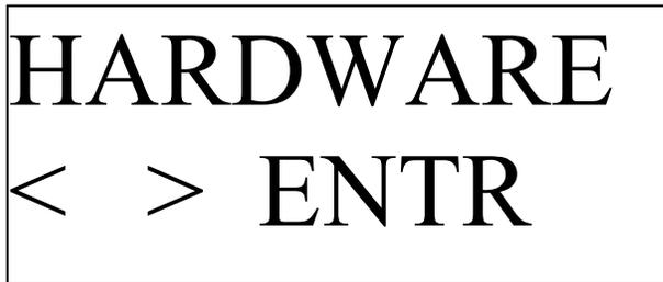
This menu allows you to change the handshaking protocol between “HARDWARE” and “XON/XOFF” for software handshaking. This menu is only available if YES is selected in the SERIAL:Y menu.
