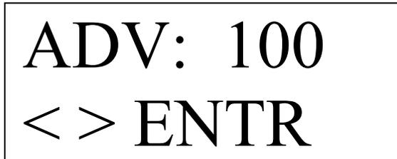
This menu allows you to “ADVANCE” the material a specified length while plotting. Material advance length setting sent by your computer software may override setting made at the keypad. This feature is useful in improving media tracking of plotter. The number display is in plotter current unit, which is either Inches or Centimeters
